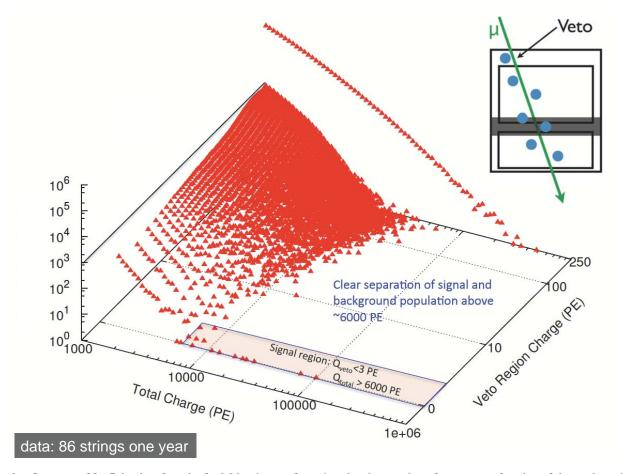
**Fig. 6** One year of IceCube data from its final 86-string configuration showing number of events as a function of the total number of photoelectrons and the number present in the veto region. The signal region requires more than 6000 photoelectrons with less than three of the first 250 in the veto region of the detector. The signal, including nine events with reconstructed neutrino energy in excess of 100 TeV, is clearly separated from the background.
