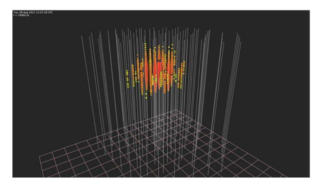
Fig. 5 Light pool produced in IceCube by a high-energy neutrino. The measured energy is 1.07 PeV, which represents a lower limit on the energy of the neutrino that initiated the shower. The vertical lines of white dots represent the sensors that report any detected signal. Color of the dots indicates arrival time, from red (early) to purple (late) following the rainbow. Size of the dots indicates the number of photons detected.
