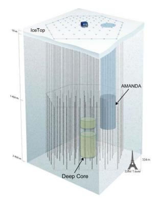
Fig. 4 Schematic of the IceCube detector.
