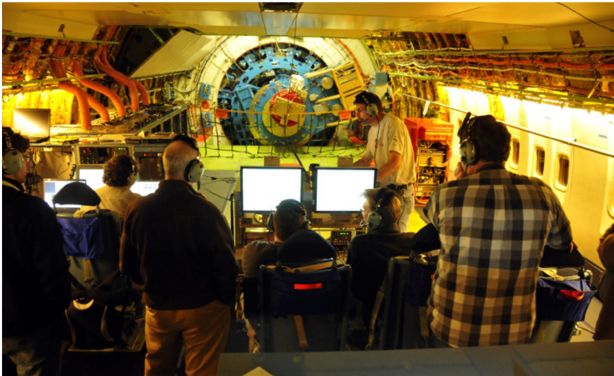
Fig. 4 Working environment onboard SOFIA during the first early science flight with FORCAST. Terry Herter (center right, in charge, standing at the PI rack). The FORCAST instrument is mounted at the Nasmyth focus and the telescope counterweight structure can be seen at the far end at an elevation angle of about 20 degrees. Photo USRA gallery.
