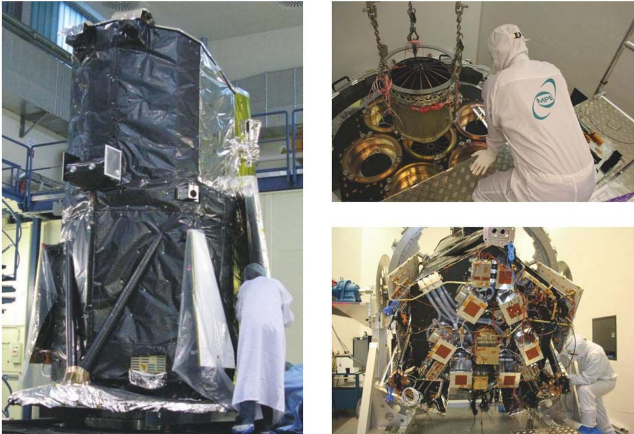
**Fig. 6** At the end of 2012, the complete eROSITA telescope underwent its qualification program (*left*, during the preparation of the thermal vacuum test). Afterwards, the instrument was disassembled in order to check for damages and failures (*upper right*, removal of the central mirror module). For the qualification, the instrument was equipped with one camera and six mass dummies (*lower right*, showing the seven modules together with the complete thermal system).
