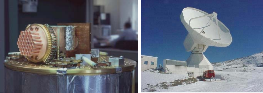
Figure 1: Left: The Max-Planck Millimeter Bolometer “MAMBO”, a 37-element array bolometer sensitive to radiation with wavelengths from 1.0 to 1.4 mm (Kreysa et al. 1999). The opened cryostat reveals the 5 mm diameter feed horns that collimate the incident radiation onto germanium semiconductor elements, which are cooled to 0.3 K. Right: The IRAM 30 m telescope on Pico Veleta in the Spanish Sierra Nevada.
